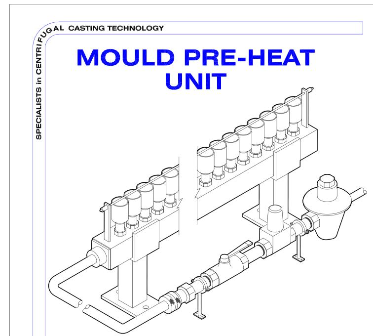
A typical system for pre-heating moulds on horizontal centrifugal casting machines.
